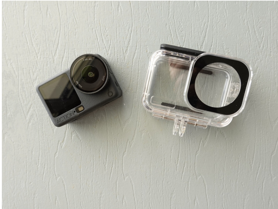
The Action 6 beside the clear Telesin 60 m housing, showing the tempered-glass port and filter-ring bezel.
